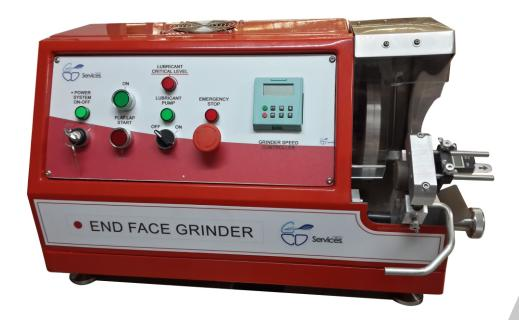
The End Face Grinder (PCT-100) allows polishing the surfaces of each core plug sample with an accuracy of 0.01 mm to rectify those plugs after Trimming process with imperfections.
