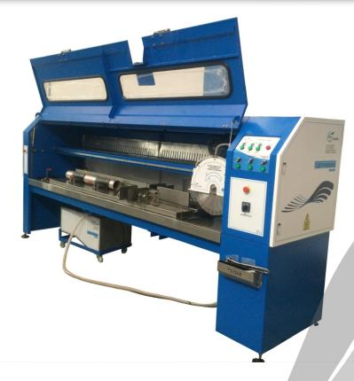
The core saw is a powerful tool in the process of analyzing samples, after a cut it leaves an excellent surface to make detailed descriptions and take photographs. It's powerful engine of 7.5HP and one diamond blade of easy change, (which brings a special grooving that optimizes the cutting process) achieve as mooth surface for the following analysis.
